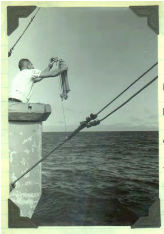
Al Smith putting Nansen Bottle on the line for a deep cast.
